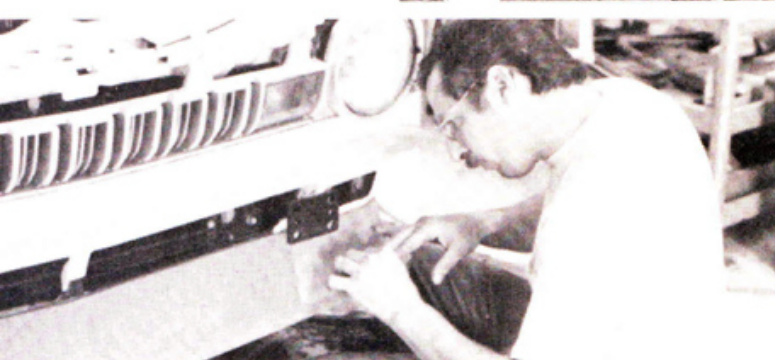
For 1977, a trick Opel Isuzu is possible; shown here is projected air dam taking shape under Larry Turk.
